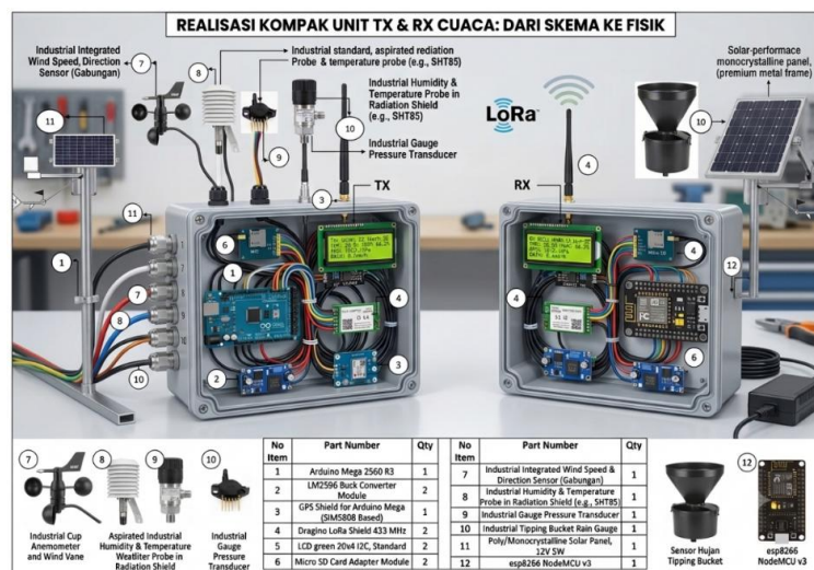
Figure 6. Componen Inside Mini AIS with Weather Sensor
